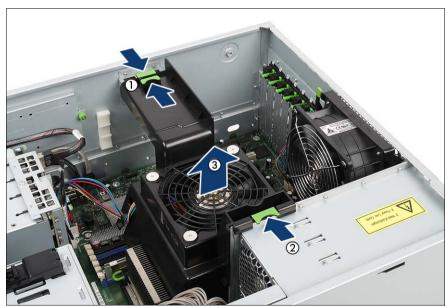
Figure 29: Example: Removing system fan 2&4
